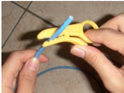
Figure 11: Stripping the cable jacket
